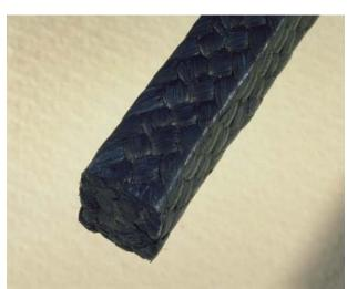
An exceptional packing combining highpurity carbon, micro-fine wires of Inconel® and a lubricant of selected non-migratory graphite to produce a product for sealing valve glands in high pressure and high temperature applications.
