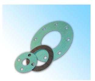
An economic grade based on a mixture of aramid and glass fibres with a nitrile rubber binder. Suitable for general industrial service including oils, hydrocarbons, low pressure steam and water.
