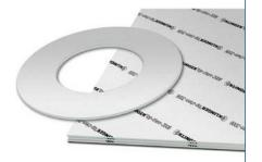
TOP-CHEM 2006, a PTFE-based gasket filled with Barium sulphate, offers resistance in strong alkaline applications and good mechanical properties.
