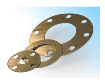
Klinger Milam is an asbestos free sealing material based on mica reinforced with stainless tanged insert. It is specifically designed for hot, dry gas applications 1000°C. to However, up outstanding chemical resistance of mica makes the gasket suitable for a wide range of applications.
